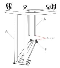
2. Arrange the appropriately marked leg with the coordinating side of the beam. Slide the bases over the vertical plates on each side of the beam. Align the holes on the legs with the holes in the beam. Attach the bases to the beam by inserting round washer head screws through long side of the columns, hand-tighten them.
