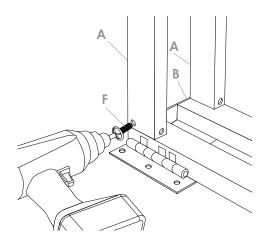
**3.** Use either #3 Phillips screwdriver or impact drill with #3 Phillips bit to tighten bolts as much as possible.
