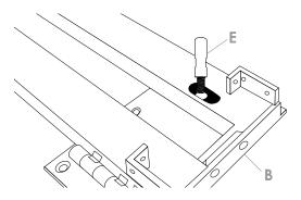
1. Lay the beam upside down on a piece of cardboard or carpeted surface. Remove the release rod from the hardware pack, and screw it into the beam.
