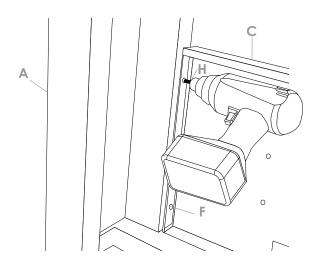
**4.** To attach the modesty panel, position the top flange on the beam and align the holes on the side flanges with the holes in the columns.
