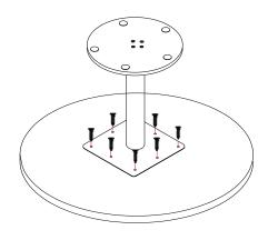
ATTENTION: <u>Due to sensitive nature of the stainless</u> steel, use extreme care when assembling a base to avoid accidental dents and scratches.
