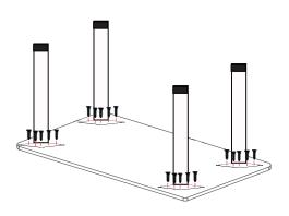
ATTENTION: <u>Due to sensitive nature of the stainless</u> steel, use extreme care when assembling a base to avoid accidental dents and scratches.
