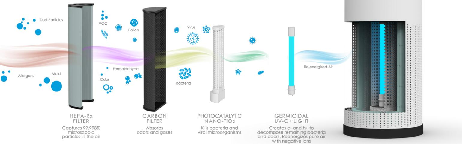
As the air is drawn through the bottom of the unit, it passes through the HEPA-Rx Filter, the Activated Carbon Filter, and the Germicidal UVC+ Photocatalytic Nano-TiO<sub>2</sub> chamber. At the final stage, the purified air moves through the Revitalizing Negative Ion Generators near the air outlet and releases negative ions into the air.
